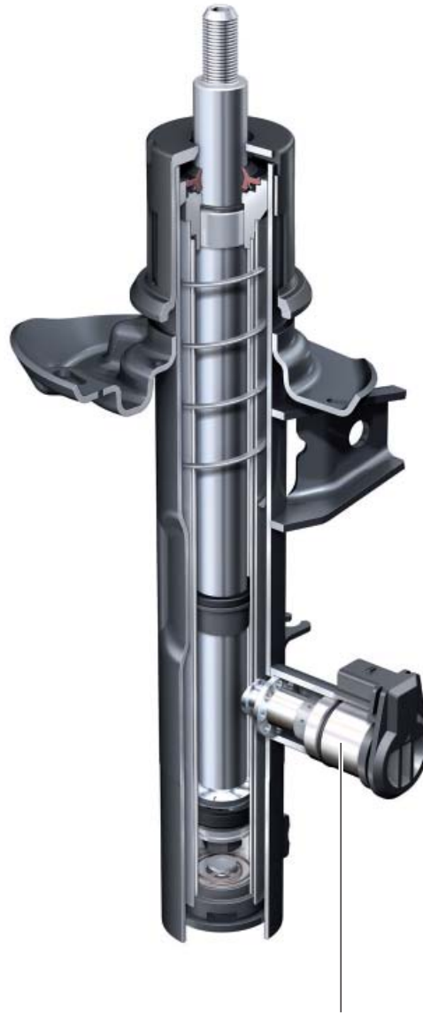
Electrically activated solenoid valve (damping adjustment valve)
